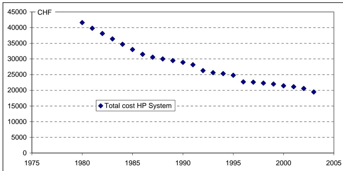
*Figure 4* Estimated total cost development of HP systems using vertical borehole as a heat source (example new single family house, including drilling and installation costs). Source: FWS (2008).
