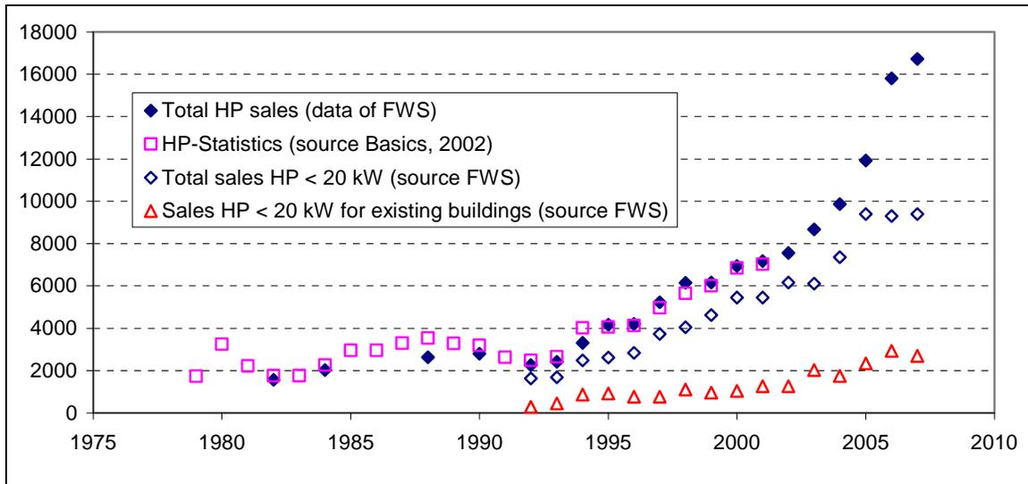
Figure 2 Sales statistics of heat pumps in Switzerland 1982 – 2006 (all types of heat pumps). Based on data from Swiss Heat Pump Promotion Group (FWS, 2008) and (Basics, 2002)
