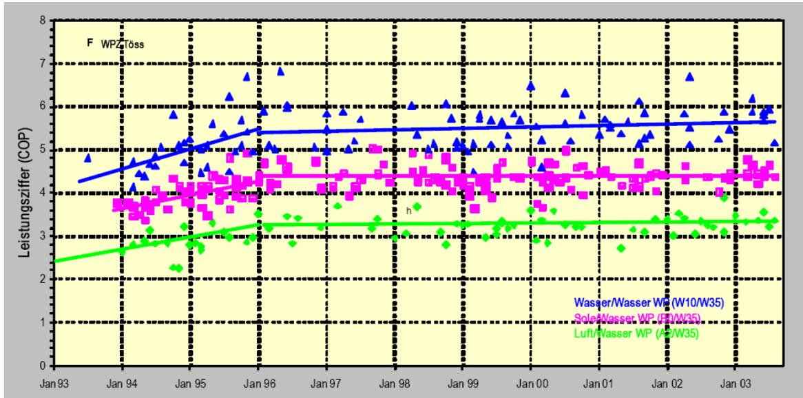
*Figure 3 Development of measured Coefficient Of Performance (COP) at Töss Test Centre in Switzerland. Source: WPZ-Bulletin [translations: Wasser: water, Sole: brine; Luft: air; Leistungsziffer: coefficient of performance]*
